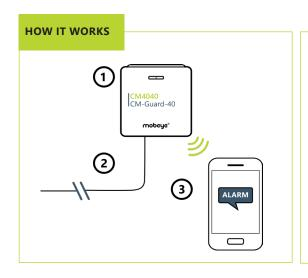
The Mobeye CM4000 monitors your installation remotely. The alarm device immediately sends a notification when the status changes, wit a clear indication which input is involved.
