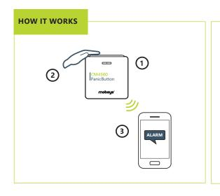
The Mobeye CM4500 is triggered after pressing the button. The panic alarm instantly sends a notification to predefined contacts. This provides extra security in vulnerable situations.
